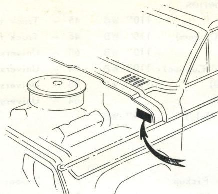
This 13 digit number can be found stamped on the bottom line of the metal plate which is affixed to the upper left corner of the firewall under the hood. Beginning with SIX DIGIT Serial Number 100000 the "Alphabetical" GVW rating code is replaced by the actual "Numerical" weight designation.
