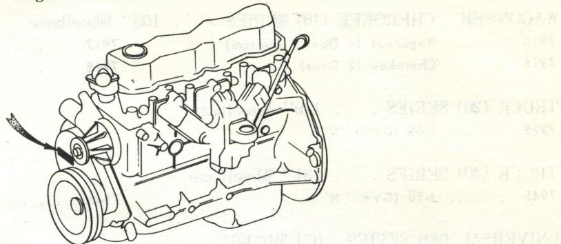
The Engine Build Plate has a code stamped on it and shows the type of engine and the date the engine was assembled.
